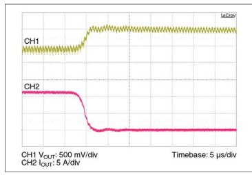
**Figure 16** — 10 A – 0 A transient response:  $C_{IN} = 100 \,\mu\text{F}$ , no external  $C_{OUT}$
