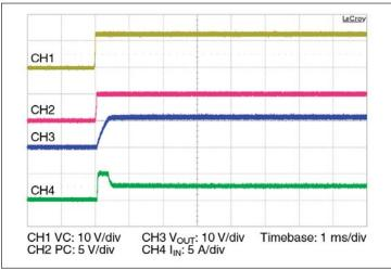
**Figure 14** — Start up from application of VC;  $V_{IN}$  pre-applied  $C_{OUT} = 500 \ \mu F$
