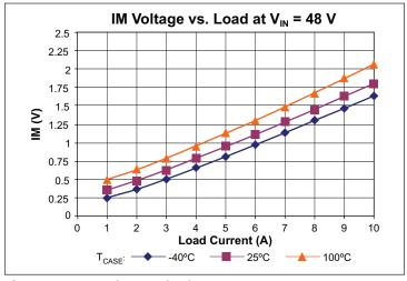
Figure 8 — IM voltage vs. load
