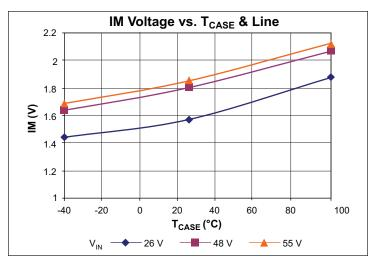
Figure 10 — Full load IM voltage vs. TCASE
