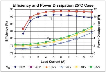
Figure 4 — Efficiency and power dissipation at 25°C
