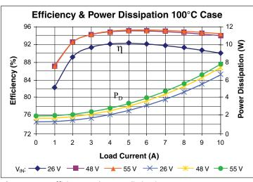
**Figure 5** — Efficiency and power dissipation at 100°C
