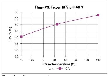
**Figure 6** — R<sub>OUT</sub> vs. temperature
