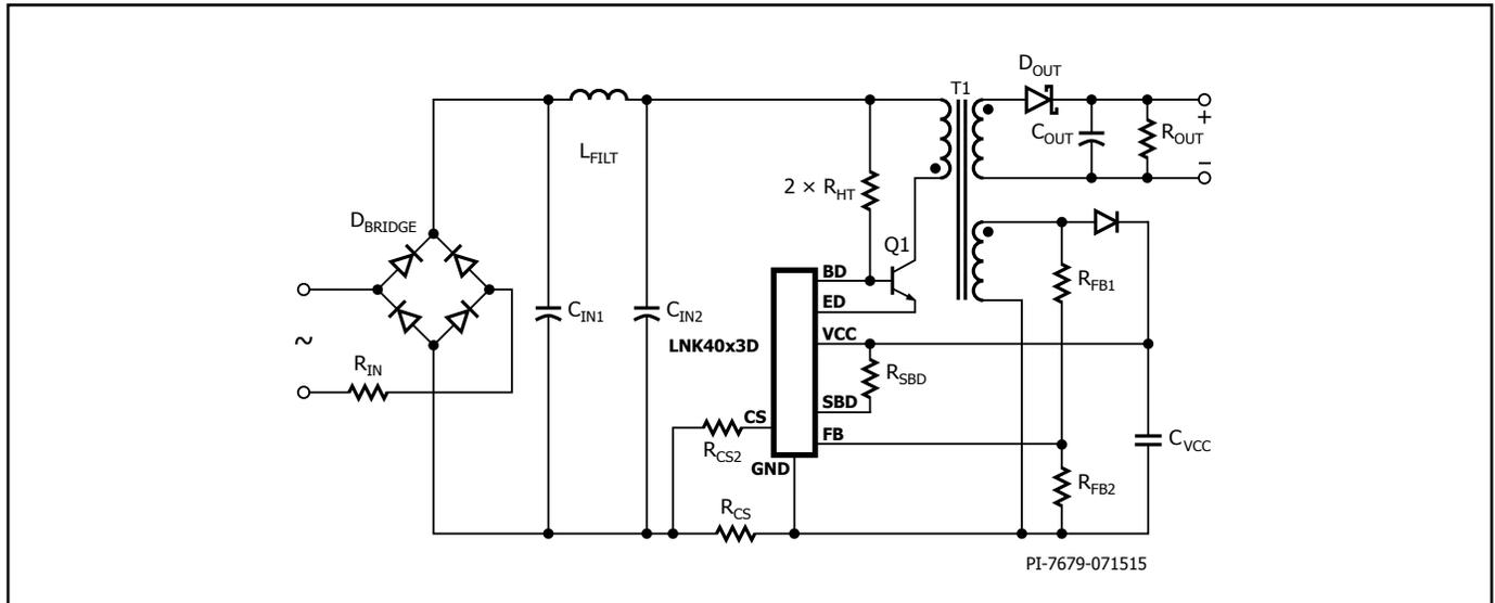
Figure 10. Typical Universal Input, 10 W Charger.
