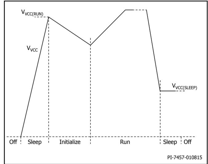
Figure 7. VCC Waveforms.
