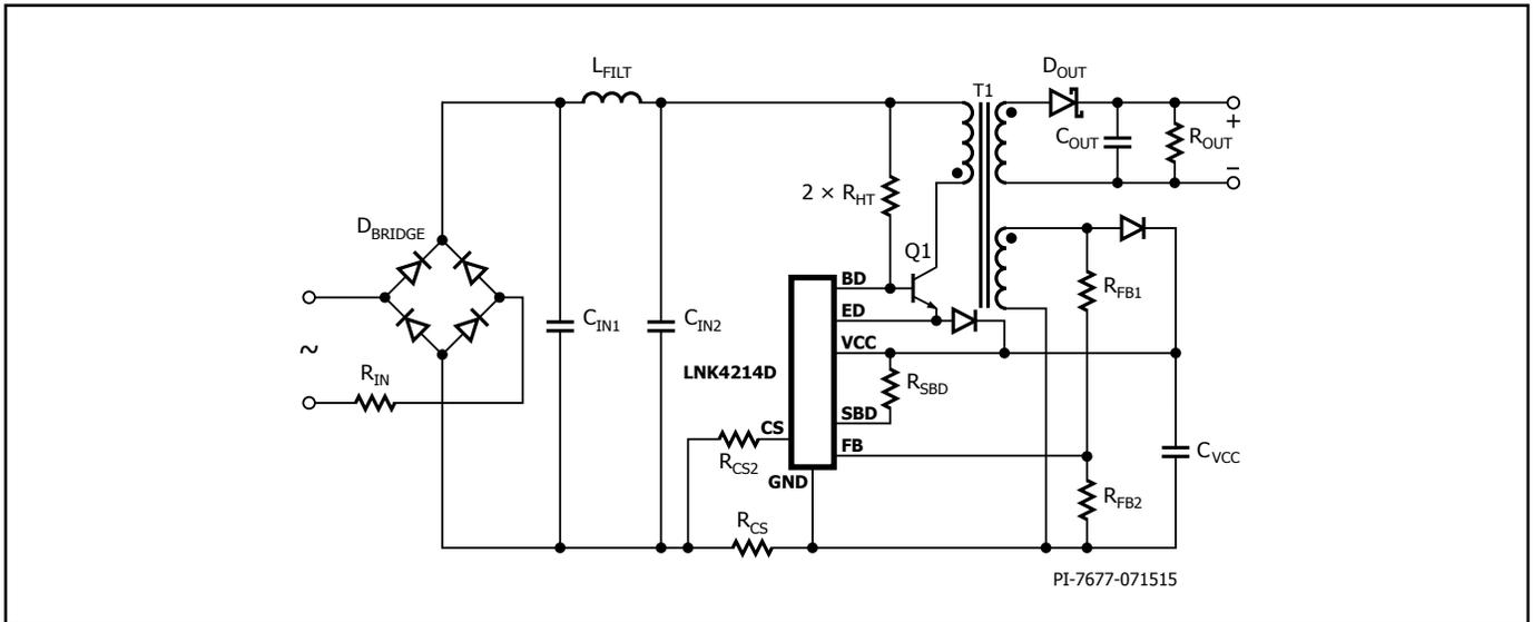
Figure 14. Typical Universal Input, 12 W Adapter.
