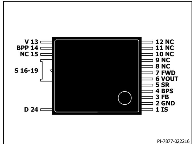
Figure 5. Pin Configuration.
