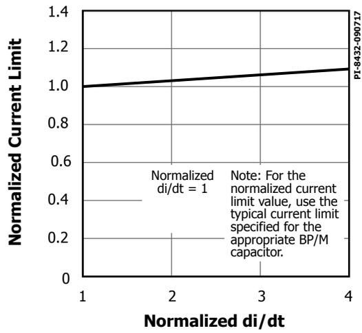
Figure 27. Standard Current Limit vs.  $di/dt$ .
