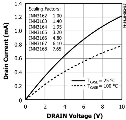
Figure 22. Output Characteristics.
