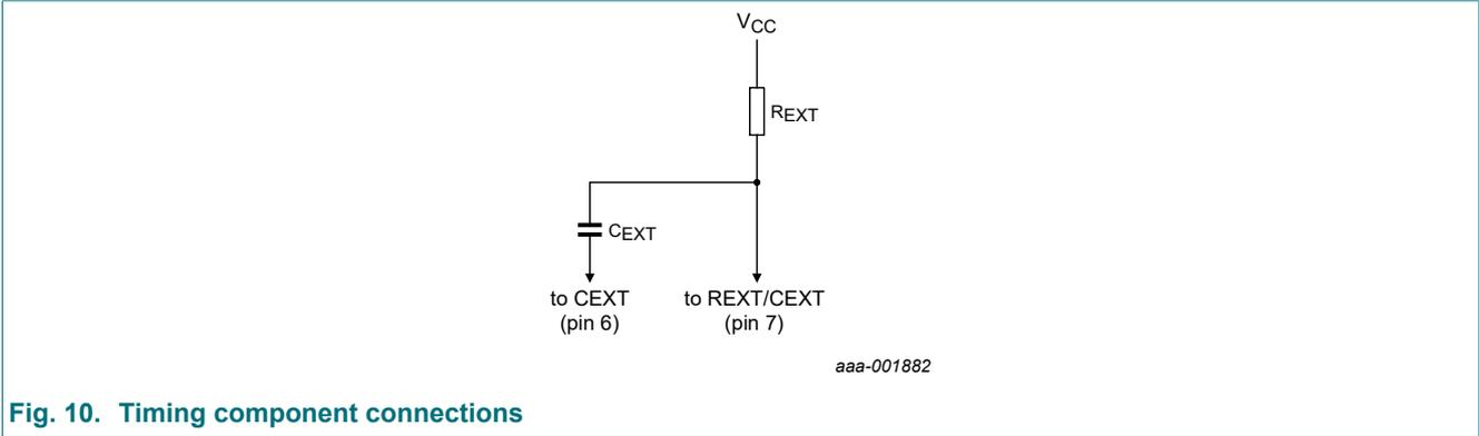
Fig. 10. Timing component connections
