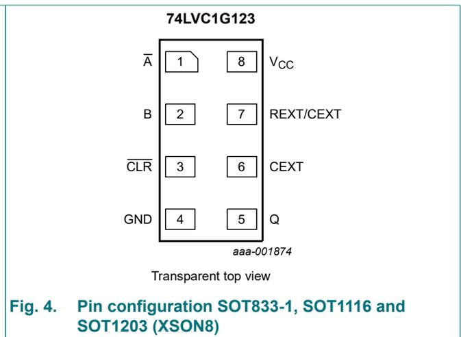
Fig. 4. Pin configuration SOT833-1, SOT1116 and SOT1203 (XSON8)
