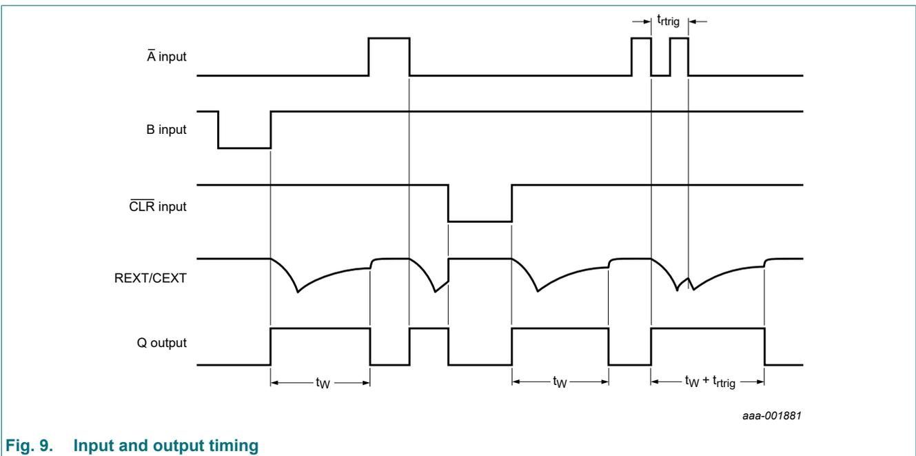
Single retriggerable monostable multivibrator; Schmitt trigger inputs
