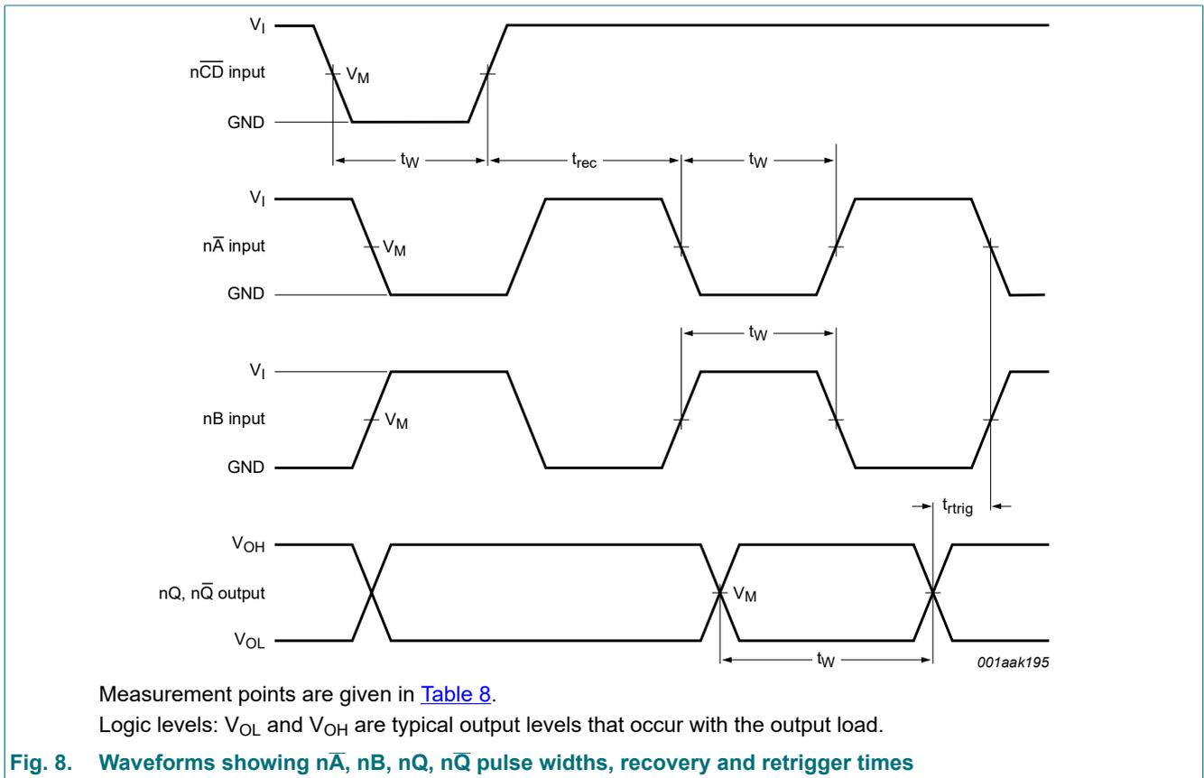
Fig. 8. Waveforms showing  $n\bar{A}$ ,  $nB$ ,  $nQ$ ,  $n\bar{Q}$  pulse widths, recovery and retrigger times
