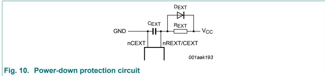
Fig. 10. Power-down protection circuit
