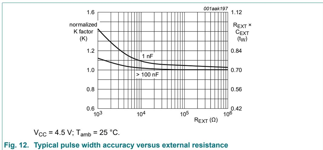
Fig. 12. Typical pulse width accuracy versus external resistance
