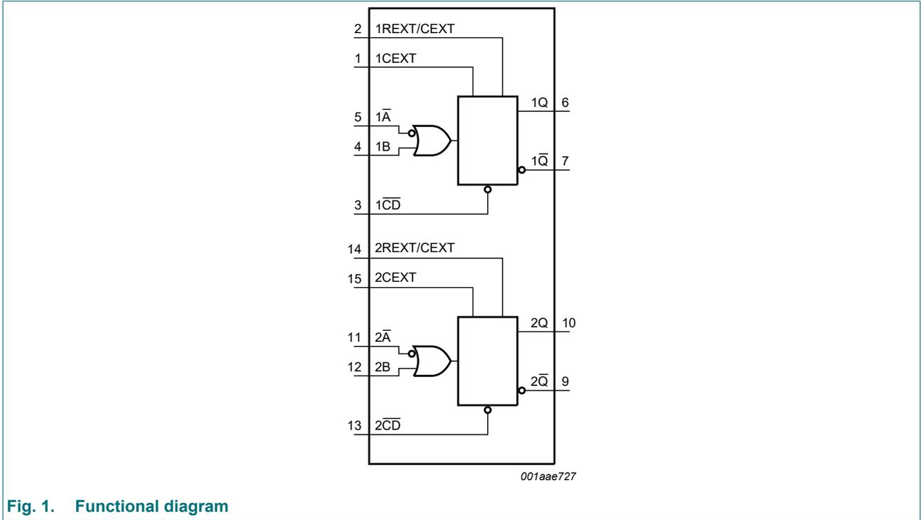
Fig. 1. Functional diagram
