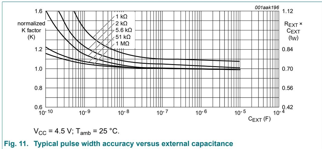
Fig. 11. Typical pulse width accuracy versus external capacitance
