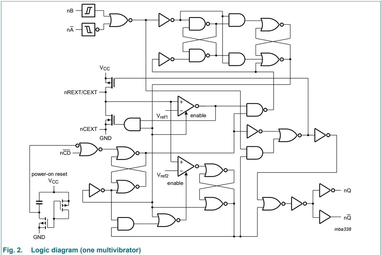
Fig. 2. Logic diagram (one multivibrator)
