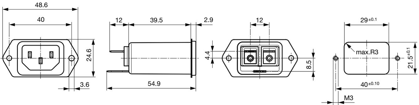
Front side mounting with plastic flange
