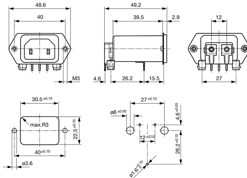
PCB rear side mounting, protection class II
